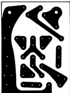
fig. 6. Printed circuit for the 1-mA S-meter. Component layout is shown in fig. 5.
