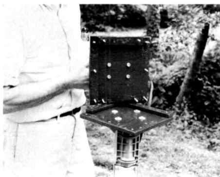
fig. 2. Details of sandwich made of 1/2-inch (13mm) plywood, well painted against weather. Bottom plate bolts to mast support for TR-44 or Ham-M rotor. Top plate bolts to U-100 rotor. Bolts fasten plates together, separated by four plywood spacers. Dimensions are shown in fig. 3.
